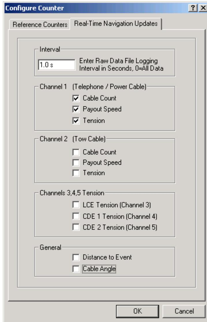
This dialog has two tabs. The first, **Reference Counters**, does not apply to this counter and should be left at the defaults. The second, **Real-Time Navigation Updates**, enables or disables this device's data from being passed to the vehicle. The three values available from this device are placed into channel one. (Channel one is reserved for product cable and is where the cable model looks for its required data.) Uncheck all remaining values, as this counter does not read them.
